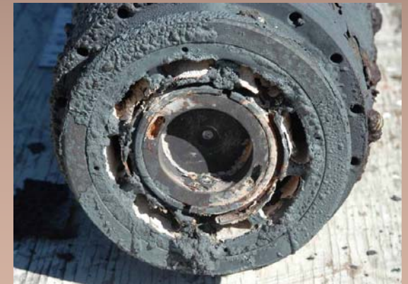
BLU-111 after FCO with Vented Base Plate
